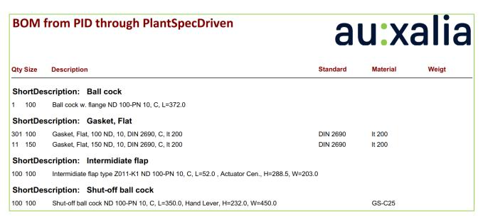
Some customers go even so far as to insert P&ID symbols like couplings, nipples, and tees in their drawings to create a Bill of Material which is used for the procurement process of the project.
