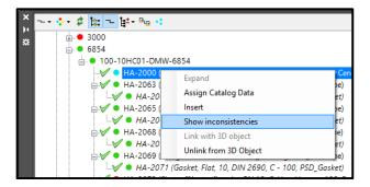
Besides checks, like Tag or Catalog data between P&ID and 3D you can define your own checks of what you would like to have checked between P&ID and 3D.
