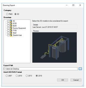
Exports P&ID and 3D drawing as standard AutoCAD® DWGs with standard AutoCAD® objects. This function will also purge the drawing and considers XREFs.
