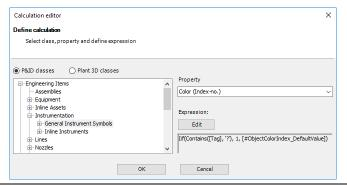
Here the color of an instrument is "calculated".
