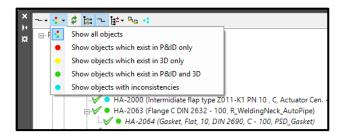
Inconsistencies can be shown just for one object, but also for the whole project. In addition, you can filter the tree for any inconsistencies.
